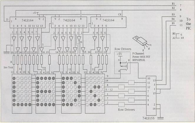
Figure II: The LED Matrix Display
